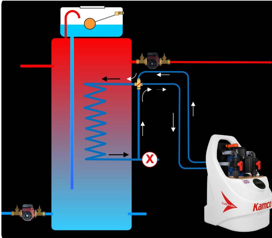
5. Attach the adaptor to the BoilerMate - two unions and washers.
